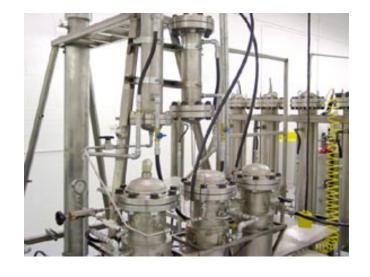
Pilot Plant Supercritical Fluid Extractor
