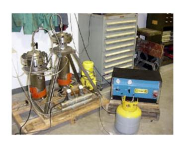
High pressure extractor configured for CO2 and compressed gases. ( refrigerants, propane, butane, etc.)
